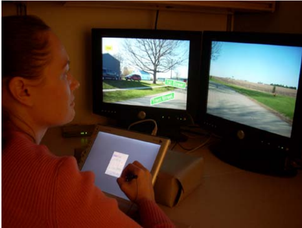
Figure 9: The computer set up included tablet PC that was situated directly in front of the user and two 20 inch monitors that were 25 inches in front of the user.
